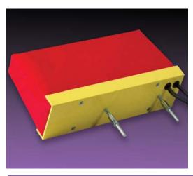
**SE-C Custom Sensing Bumpers** are designed to fit specific application needs. When deformed by contact or impact, they provide a signal in the form of an electrical contact closure. They have a large, compliant surface that helps protect personnel and equipment from injury or damage. The nylon-reinforced exterior housings are resistant to water, oil, hydraulic fluids, and coolants. Mounting options include studs and threaded holes.
