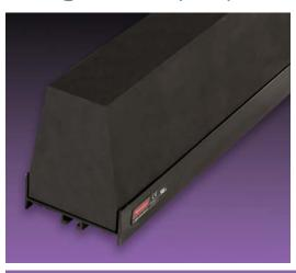
**SE-45 & SE-75 Sensing Bumpers** are designed for general-purpose, heavy-duty applications. When deformed by contact or impact, they provide a signal in the form of an electrical contact closure. At the same time, the large, compliant surface and substantial overtravel cushioning helps protect personnel and equipment from injury or damage. Operating force is 20lbs nominal.
