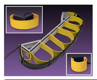
The VB-Series High-Impact Sensing Bumpers are designed to survive repeated crushing impacts that would destroy conventional bumpers, and to continue functioning perfectly. When deformed by contact or impact, they provide a signal in the form of an electrical contact closure. They are suitable for use on AGVs, mobile platforms, traveling conveyors, and other moving equipment or machinery. Sensitivity is uniform over the entire bumper surface, including any curved areas.
